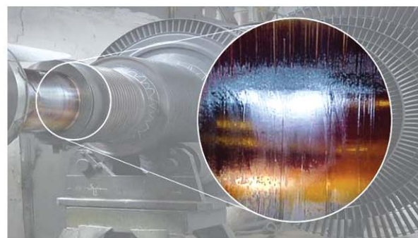
Varnish on Turbine Bearing
