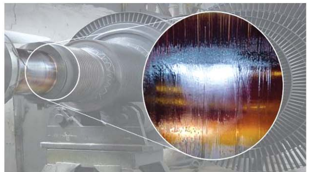
Varnish on Turbine Bearing
